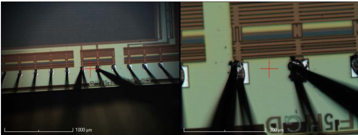
Figure 18. Power supply section of chip under test
